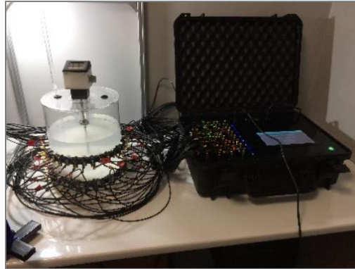
Fig. 5 View of the test stand. On the left side is the reactor model with electrodes, and on the right side there is a tomograph
