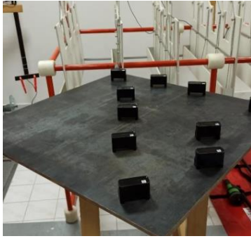
Fig. 4. Metal plate as zero potential plane for the simulation of partial discharges in HV laboratory and arrangement of the tested devices.
